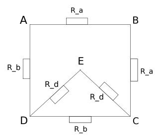
We can now imagine that one of the nodes is actually composed of 2 nodes, connected with a perfectly conducting wire (which is basically a power source with 0 potential difference) - we can also imagine that we cut the circuit at a node and connect the cut points with a wire. So, we have a source (the added wire) and a load connected to it, whose impedance is (when cutting
